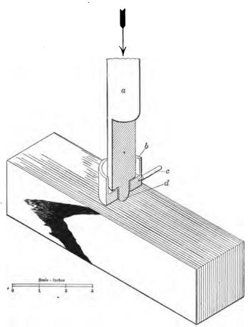
Fig. 7.—Method of making test for hardness.
